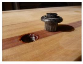
Remove the original vent and drill a 5/8" hole for the retrofit plastic vent plug. Trial fit the vent in the hole. It should be snug but not tight. Apply generous coating of epoxy to the sides and press the plug into the hole. Wipe off excess epoxy and hold the plug down with a weight until the epoxy cures.
