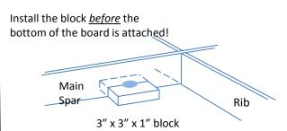
Notch main spar and glue wood block to the back of the deck with half of the block on each side of spar as shown. Drill the hole through the deck and through the block a with the hole extending into the spar. This will make an opening on each side of the spar so both sides of the board can yent.
