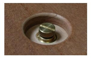
Create a recess in the deck of the board so the top of the vent screw is even with the top of the deck.
